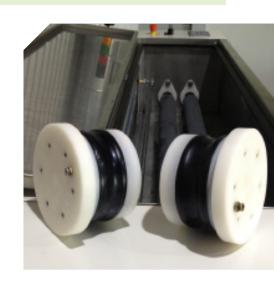
All the moving parts and drives of the nozzels is separated from the washing tank -> because it is not in direct contact with the cleaning agent there is less cleaning, maintenance and repair to do.
