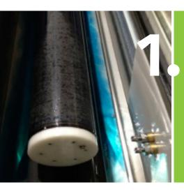
With our unique system with 2 rubber rollers at the bottom of the cleaning tank where the anilox is rotating on top, we reach a perfect cleaning result, because the cleaning agent is not only dripping of the roll surface with only little time for weakening the dried ink in the cells – but it is sprayed between the anilox surface and the rubber rollers.
