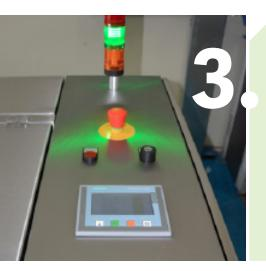
We have 3 cycles – washing with chemcial agent, rinsing with high pressured water and drying with pressured air. All 3 cycles are fully automatic and you only have to push one botton to start the machine. When the procedure is done – the machine shows an optical signal to understand that it is ready for the next roll. Of course you can programm cleaning and cycle times depending on the situation with each anilox.
